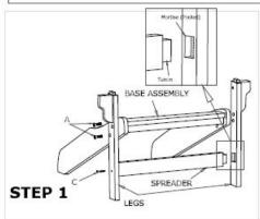
Attach Spreader tenon into mortise (pocket) on Leg Assemblies and attach with screws (C) as shown. Bolt legs to Base Assembly using bolts (A).
