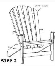
Tenons on the Back Assembly will fit into mortise (pocket) in Base Assembly, Attach with Screws (C) as shown).
