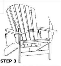
Attach Arms to front Legs from the top using screws (B). Bolt Arm Assembles to Back Assembly using Bolts (A) as shown.
