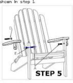
5. Attach Arm Rest Assebles using Bolt (A) with washer (E) between Leas and A Rest connection point.
