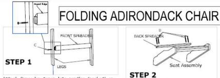
Attach Spreader tenon Into mortise (pocket) on Leas and attach with screws (C) as shown Bolt legs to Base Assembly using bolts (A).
