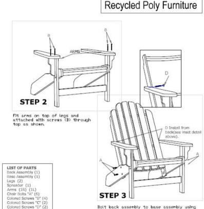
2 bolts (A) on each side as shown. Attach
