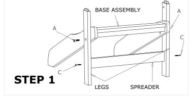
Attach Spreader to legs with screws (C) as shown. Bolt legs to base assembly using bolts (A).
