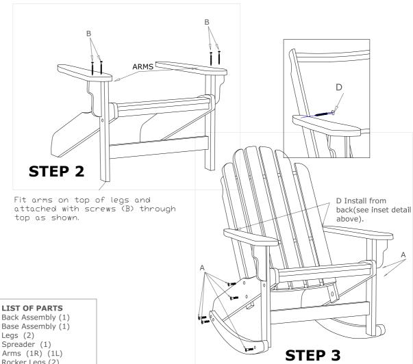
Bolt back assembly to base assembly using 2 bolts (A) on each side as shown. Attach arm to seat back using Large Head Screws (D). Bolt rocker legs to using bolt (A) as shown.
