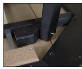
Place the table top assembly upside down on a clean, flat work surface. Position the shelf assembly with legs on top. Align the boards in the top and bottom to run the same direction. Fasten the legs to the table top assembly using two 2  $\frac{1}{2}$  screws in each leg. See photo for positioning note:  $\frac{1}{4}$  space between leg and runner.
