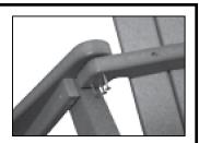
Place three 1¾" screws in the pilot holes of the back crosspiece to secure it to the back of the arm. Repeat for the other leg assembly.
