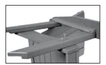
Push carriage bolts through the holes in the leg assembly. Set seat on edge. Fit the leg assembly onto the side of the seat. Tap the bolt heads with a hammer to set them firmly against the leg. Place the nuts on the bolts and tighten securely.
