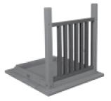
Fasten the two leg assemblies on opposite sides of the tabletop. Secure with  $2\frac{1}{2}$ " screws using the pilot holes in the legs. Fasten the side panel to the table top using 2" screws.
