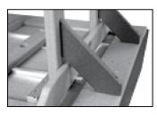
Secure each brace using two 2½" screws in the pilot holes in the legs and one 21/2" screw in the pilot hole in the brace to secure it to the tabletop.
