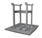
Center leg assembly on the tabletop. Fasten using 2½" screws using the pilot holes in the legs.
